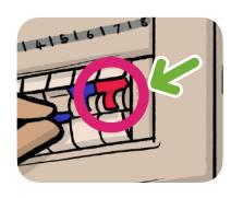
• Check the electrical safety switch in your fuse box - this is a switch that turns off the electricity in your home immediately.
